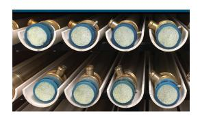
Air Liquide's membrane technology delivers uncompromising performance within a compact design. By utilizing a proven polymer blend and advanced hollow fiber technology, the unit generates an optimal balance of flux and selectivity for on-site nitrogen supply.
